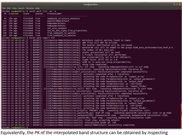
9. Equivalently, the PK of the interpolated band structure can be obtained by inspecting the output nodes of the initial workflow that we submitted (it was PK=113 in our example). This can be done by running the command verdi node show 113 and checking the PK of the output node with link label
